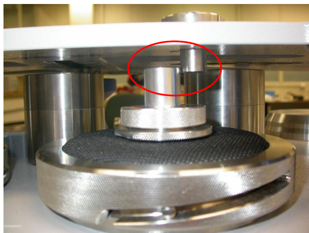
Figure A3: Contact Between Sample Holder and Spindle Guide
