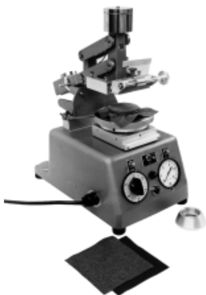
Fig. 2—C.S.I. Surface Abrader prepared for frosting test.
